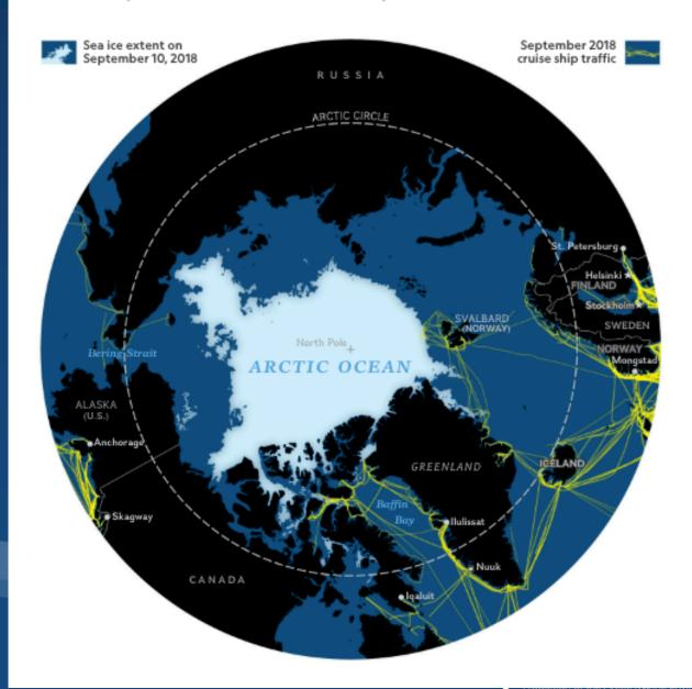
**Bulk carriers** transport materials from northern mines, such as zinc from Alaska's Red Dog mine and iron ore from Canada's Mary River Mine. Currently only accessible in summer, the ports serving these mines could be more active for longer periods as sea ice declines.
