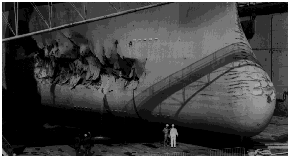
Figure 8.1. This Type D Bulk Carrier was damaged by ice in Hudson Strait. Provided by Transport Canada.
