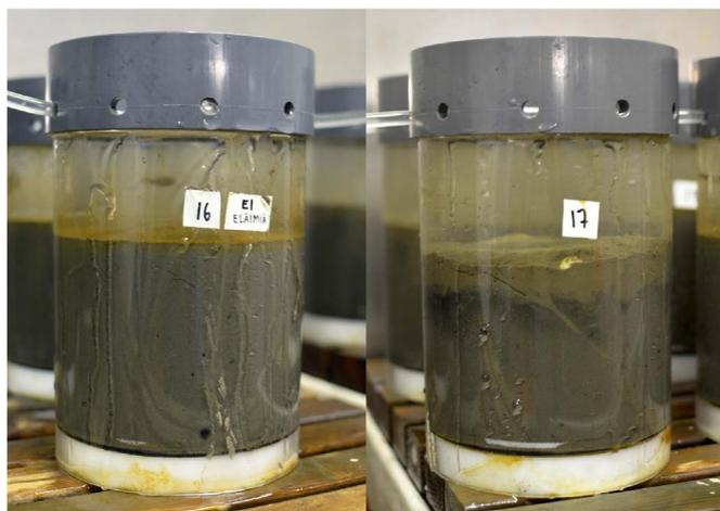
Fig. 1. Experimental cylinders at the end of the experiment; control unit (left) and unit containing animals (right). The oxidized layer is clearly visible on top of the sediment core in the animal unit, seen as lighter grey layer.
