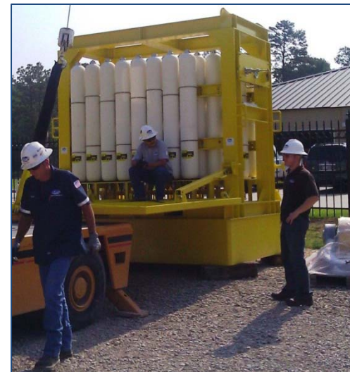
Hydraulic Accumulator Skid
