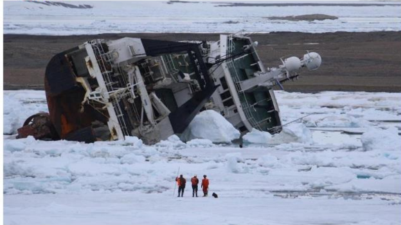
Members of the Norwegian Kystverk inspect the Northguider in July 2019. By that time ice and currents had resulted in the ship listing at larger angle than when it ran aground. (Kystverket)
